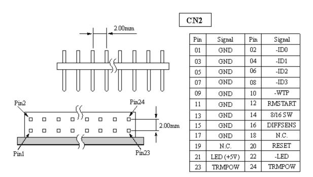
Figure 4.17 External operator panel connector (CN2)
